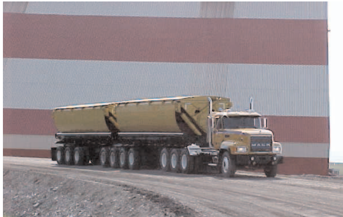
Teck Cominco has spent $16 million to address the issue of ore concentration dust since the latest study was conducted. New steel lids have been installed on trucks carrying ore to the port site, where other modifications have also occurred.
