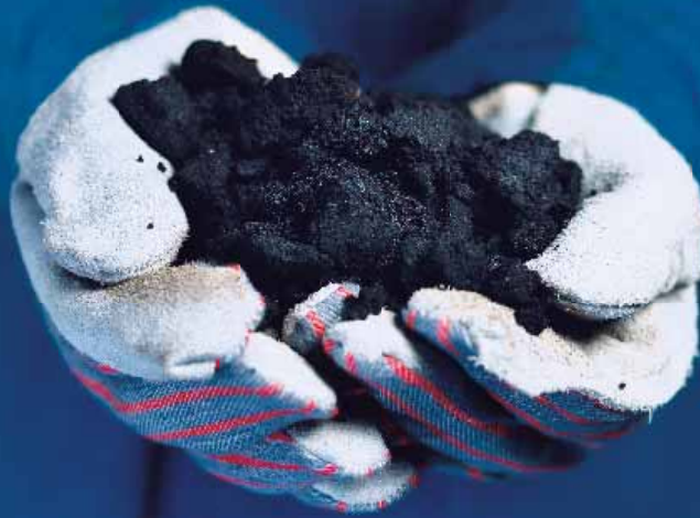
Oil Sand photo courtesy of Suncor Energy, Inc. Oil sand is a mixture of bitumen (a thick, sticky form of crude oil), sand, water and clay.
