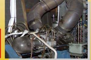
Even moderate fractions of FT fuel blended in JP-8 significantly reduce exhaust emission particulates in T63 turbine engine testing.
