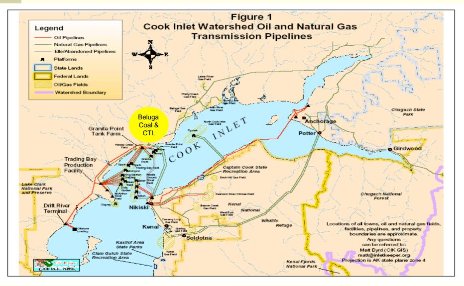
Most of the oil and gas production is from the west side of the Cook Inlet plus an inefficient simple cycle 350 MW gas fired power plant due for replacement – all within a few miles of the proposed CTL site
