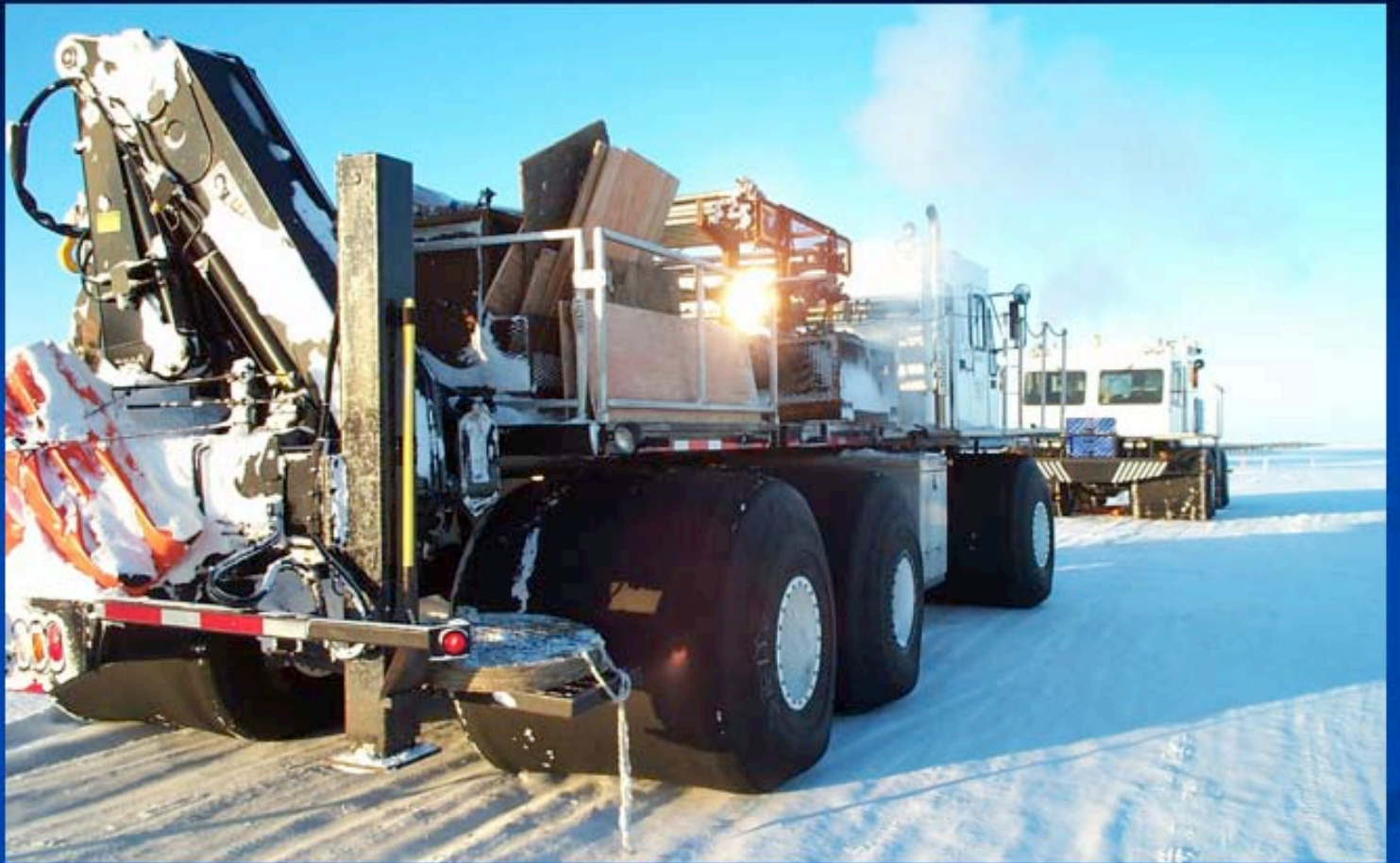
Low Ground Pressure Vehicle on Packed Snow Trail
